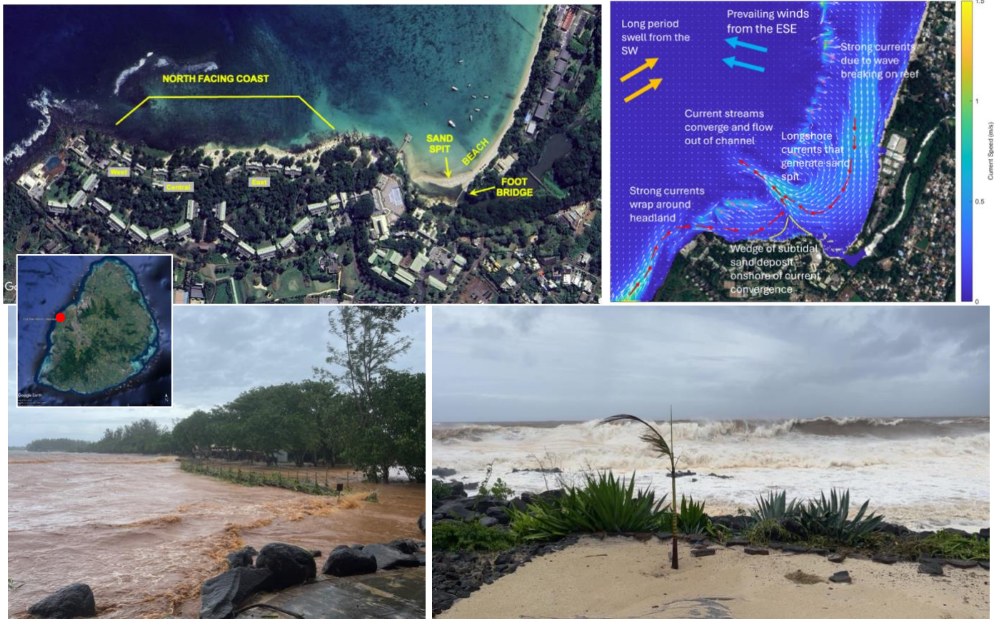
(inset) red dot shows the location of Albion (top left) the layout of the Club Med Resort (top right) numerical modelling results showing the coastal processes (bottom left and right) flooding and high waves at Albion during Cyclone Belal.
