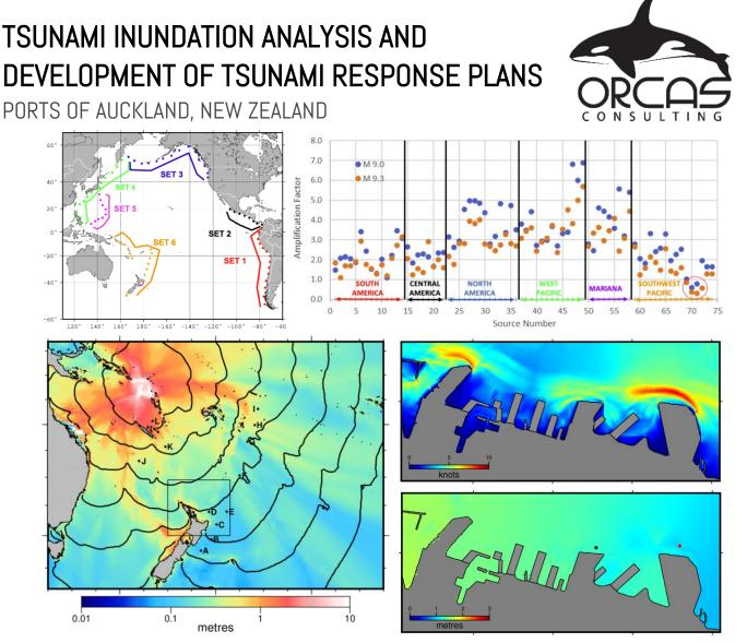
(top left) Dots indicate the locations of the 73 tsunami sources used in the analysis (top right) tsunami amplitude amplification factor inside the port of Auckland for each source. (bottom left) regional propagation for a MW 9.2 earthquake tsunami source in the Solomon Islands (bottom right) Maximum computed current speed (top) and amplitude (bottom) for that source
