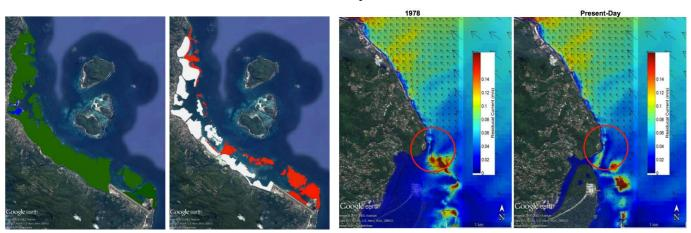
(left to right) 1978 reef areas (green) and reclaimed areas (blue). 2016 reclaimed areas (white) and reef areas (red). Comparison of residual currents on the 1978 bathymetry (left) and the present-day bathymetry (right). Note the enhanced hydrodynamic connectivity between the fringing reef and the coastline along North East Point in the 1978 which has been reversed as a result of the extensive modifications to the reef.
