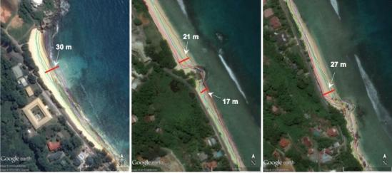
Maximum shoreline fluctuation at North East Point over the available imagery data: northern end (left) central section (mid) and southern end (right).
