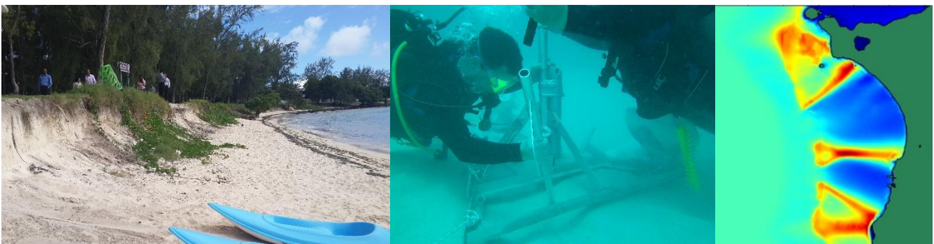
(L to R) The heavily eroded southern end of Mon Choisy; installing a wave gauge offshore; model output showing wave focussing towards the southern end of the beach, contributing to the erosion.
